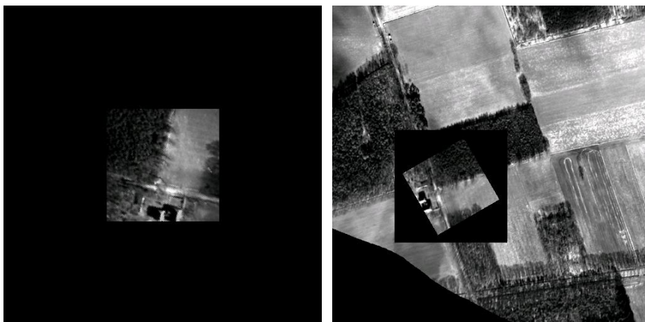
Fig. 4: (left) Scaled template a= 1.6 and rotated for 40 degrees. (right) Registered images.
